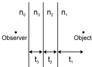
$$\text{Apparent shift} = t_1 \left[ 1 - \frac{1}{n_{1\text{rel}}} \right] + t_2 \left[ 1 - \frac{1}{n_{2\text{rel}}} \right] + \dots + \left[ 1 - \frac{n}{n_{\text{rel}}} \right]$$
