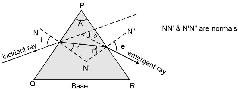
$$\delta = (i + e) - (r_1 + r_2) \text{ and } r_1 + r_2 = A$$
